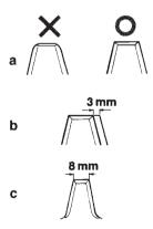
2. When sharpening, offset the teeth of upper and lower blades by 3mm. (b) To offset, insert the hexagon wrench into the socket on the top of the cuttercase and rotate it.
